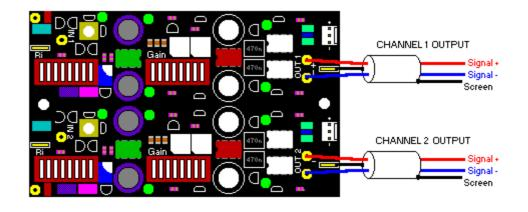
WARNING! Avoid shortcircuting any of the outputs (+ or - outputs) to ground. Also avoid connecting + and - outputs directly to each other. Doing so will damage the output devices.
