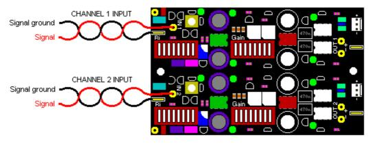
Fig. 4. Connecting the cartridge using screened cables.
