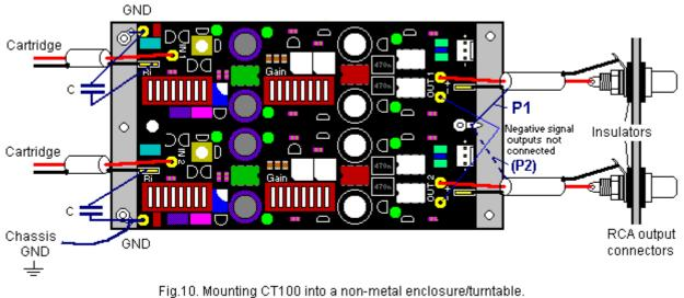
This example uses non-balanced output connections (RCA connectors)
