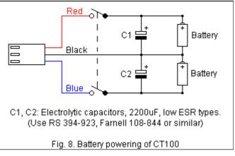
the mains when the charging is ended in order to assure all advantages of battery powering. Each CT100 is supplied with two cables terminated with locking connectors intended for connecting CT100 to batteries or other power sources. The three cores are colour coded in accordance with fig. 1. (See <u>CONNECTIONS</u>). See also fig. 8.
