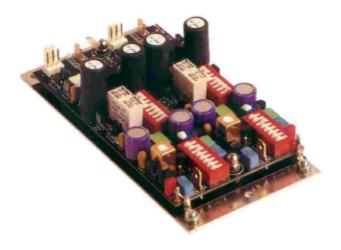
Phono preamplifier module with very accurate RIAA equalization (0.05dB).
