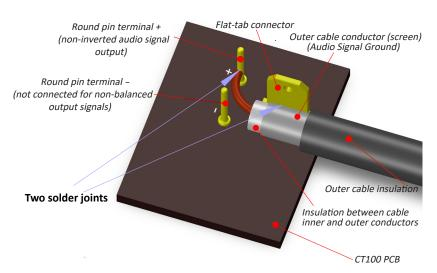
Fig. 4. CT100 audio signal output connections, non-balanced
