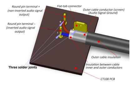
Fig. 5. CT100 audio signal output connections, balanced
